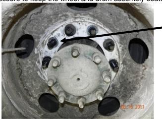
Locate 1<sup>st</sup> stud clockwise from the valve stem; install the first antiindexing sleeve. If everyone follows this procedure, you will have
