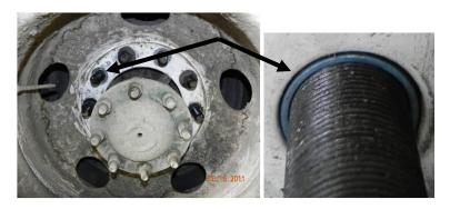
WARNING: Selecting an anti-indexing sleeve that is to long may damage the brake drum face and/or interfere with the nut's flange washer producing false or lower torque and clamp load, resulting in the wheel(s) loosening or separating from the vehicle causing; property damage, injury, even death.
